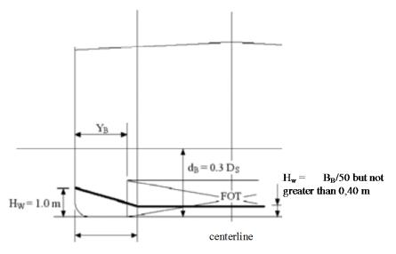
B<sub>B</sub>/5 or 11,5 m, whichever is less (measured inboard from the ship's side at right angles to the centreline at the leved of d<sub>B</sub>)
